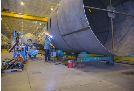
**Top:** Team has standardized its welding booths with the Miller PipeWorx 400 welding system, which fits the company's varied welding requirements. The single-system design with one machine footprint helps maximize weld cell space.
